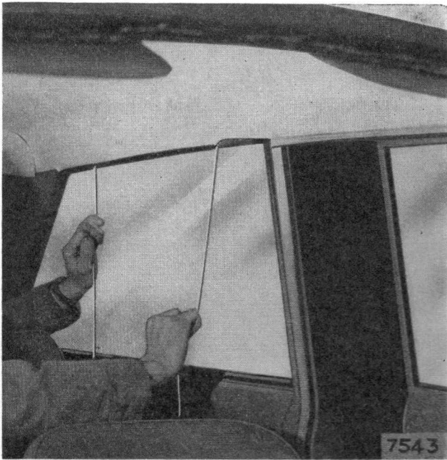
Fig. 9. Fitting rear quarter glass
