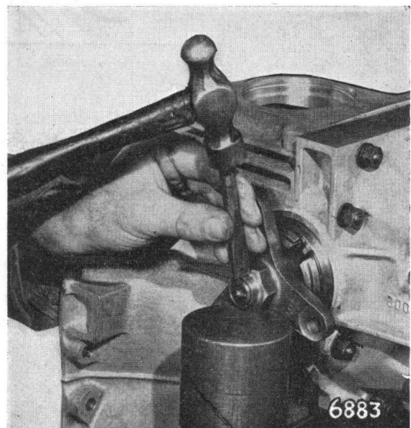
Fig. 46. Peening drive flange nuts
