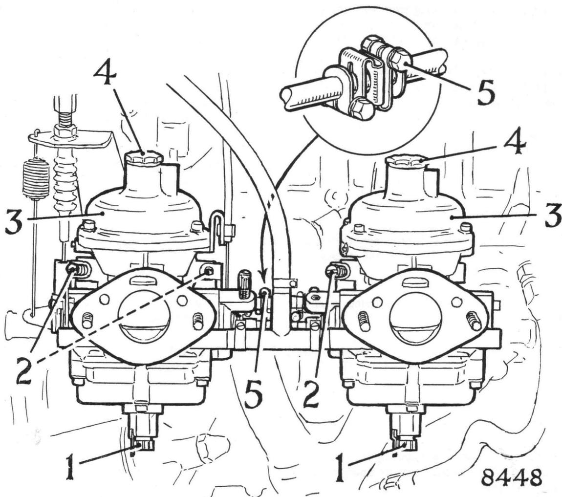
Fig. 8. Throttle synchronisation and jet adjustments
