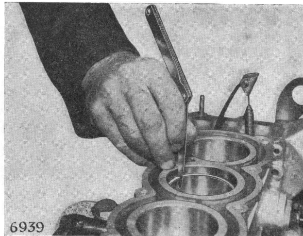
Fig. 47. Checking piston ring gaps
